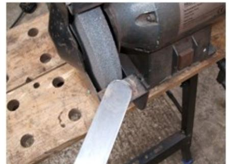
Then I use a Grinding disc, in the Angle Grinder to grind off the sharp corners from all around the sword. When I have a basic rounded edge all around the swords I then move to a Linisher machine or (belt sander) to complete the rounding of all the edges on each sword blade.
