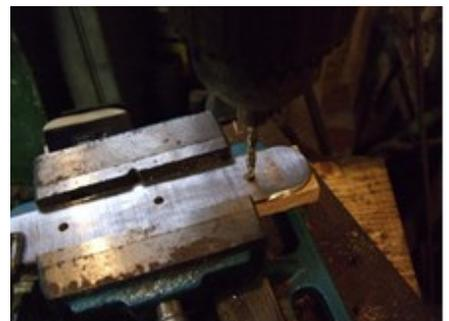
When both handles have been drilled and countersunk assemble the handles to the blade, put the rivets in place, cut the rivets to the correct length to allow for riveting over into the countersink of the handle. When ready put a drift or round bar the size of the rivet head in the vice, and rivet the end of the aluminium rivet into the countersink of the handle with a ball peen hammer.
