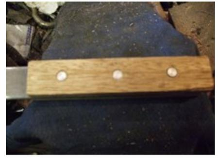
When the wooden handles have been riveted onto the blade, file the wood to the shape of a handle. I use a rasp to ruff out the shape and then finish the shape with a file. When you are happy with the shape of the handles use sand paper to get a nice smooth shape.
